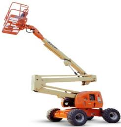
**Articulating Boom Platforms** – An aerial device with two or more hinged boom sections. They are designed to reach up and over obstacles.
